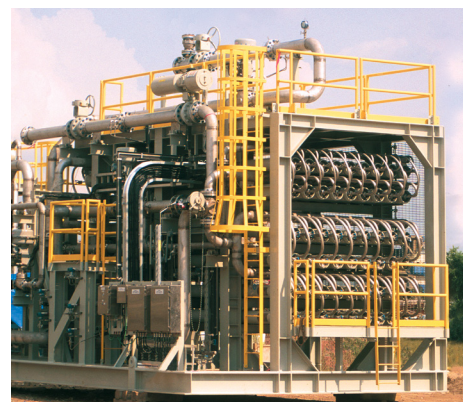
One of seven sulfate reduction modules capable of producing 50,000 bbl/d (330 m 3 /h) of low-sulfate seawater for Kizomba A Field, West Africa.
