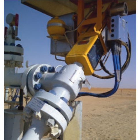
CC30 choke with linear hydraulic actuation
