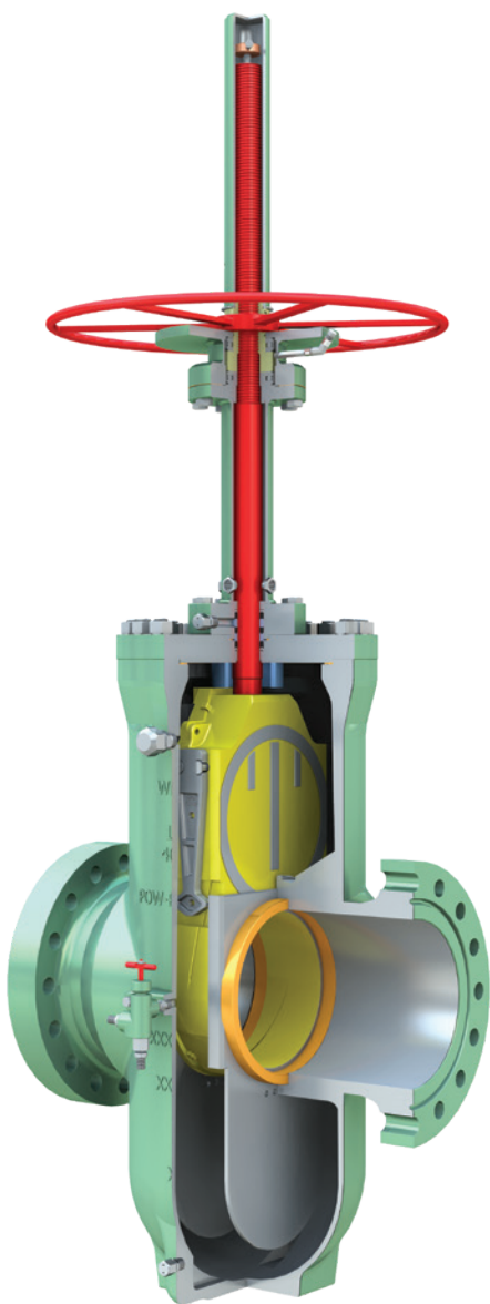
WKM Pow-R-Seal double expanding gate valve.
