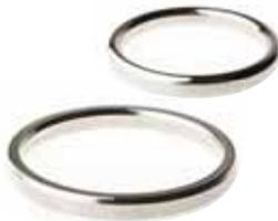
R type ring joint gaskets are available in oval or octagonal cross section and manufactured in accordance to API 6A and ASME B16.20 to suit API 6B and ASME/ANSI B16.5 flanges.
