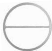
Double jacketed gaskets are completely enclosed by a two piece metal covering OD, ID and both sealing surfaces. Widely used in heat exchange applications and suitable for corrosion and high temperature service.
