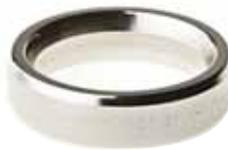
The RX type RTJ gasket is manufactured in accordance to API 6A and ASME B16.20 to suit API 6B and ASME/ANSI B16.5 flanges. The RX is a pressure energized version of the R octagonal gasket and fits the R type flat bottomed groove.
