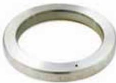
The BX type RTJ gaskets are manufactured in accordance with API 6A and are suitable for use in high pressure API 6BX flanges. The gaskets form a metal to metal seal on assembly and the efficiency improves as internal pressure increases.
