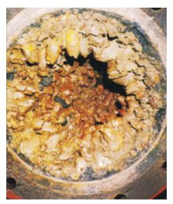
An example of a severely fouled pipe from a system without a BFCC system.
