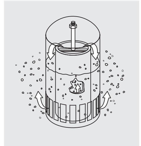
Glycol dehydration system bubble cap.
